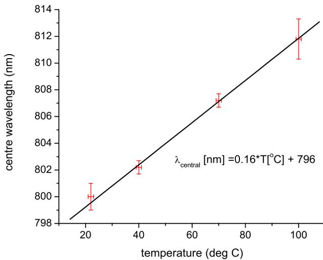
**Fig. 4** Temperature tuning of adiabatic DFG. By tuning the temperature of the adiabatic crystal over an 80°C range, the seed depletion spectrum shifts by ~12 nm, corresponding to more than 200 nm of central wavelength tunability in the mid-IR
