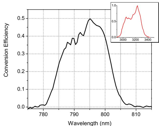
**Fig. 3** Conversion efficiency of the seed pulse for ultrafast adiabatic DFG. The peak efficiency reaches 50%, and remains high ( $\geq 35\text{--}40\%$ ) over 20 nm of seed bandwidth. *Inset*: normalized spectrum of the DFG pulse as a function of wavelength in nm
