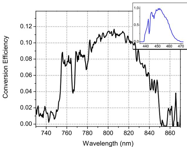
**Fig. 2** Conversion efficiency of the seed pulse for ultrafast adiabatic SFG. The efficiency curve is nearly flat over the bandwidth of the seed pulse, indicative of the robustness of the adiabatic frequency conversion method. *Inset*: normalized spectrum of the SFG pulse as a function of wavelength in nm
