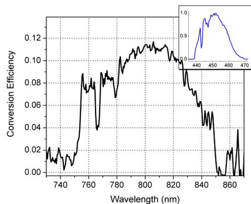
Fig. 2. Measured conversion efficiency of the seed pulse in the SFG process. Inset: normalized spectrum of the SFG pulse as a function of wavelength in nm.
