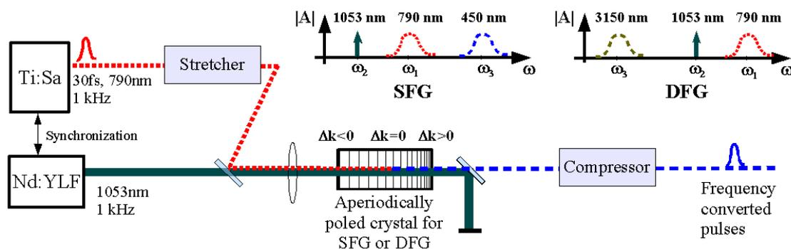
Fig. 1. Implementation of adiabatic frequency conversion of ultrafast pulses. The stretched seed pulse from a Ti:S multipass amplifier (dotted red line) and a strong 1053 nm pump beam from a Q-switched Nd:YLF laser (solid green line) are mixed in the adiabatic aperiodically poled nonlinear crystal. Depending on the adiabatic crystal design, the energy in the seed beam can be efficiently converted to either the sum frequency or difference frequency beam (long dashed blue line).
