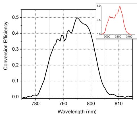
Fig. 3. Measured conversion efficiency of the seed pulse in the DFG process. Inset: normalized spectrum of the DFG pulse as a function of wavelength in nm.
