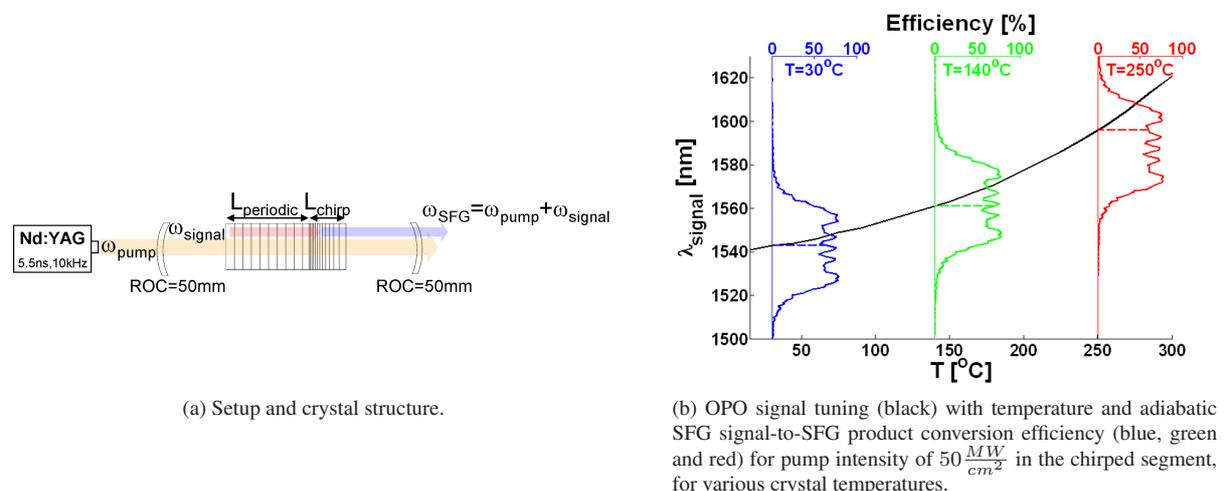
Fig. 1. Setup, crystal structure and simulation results.
