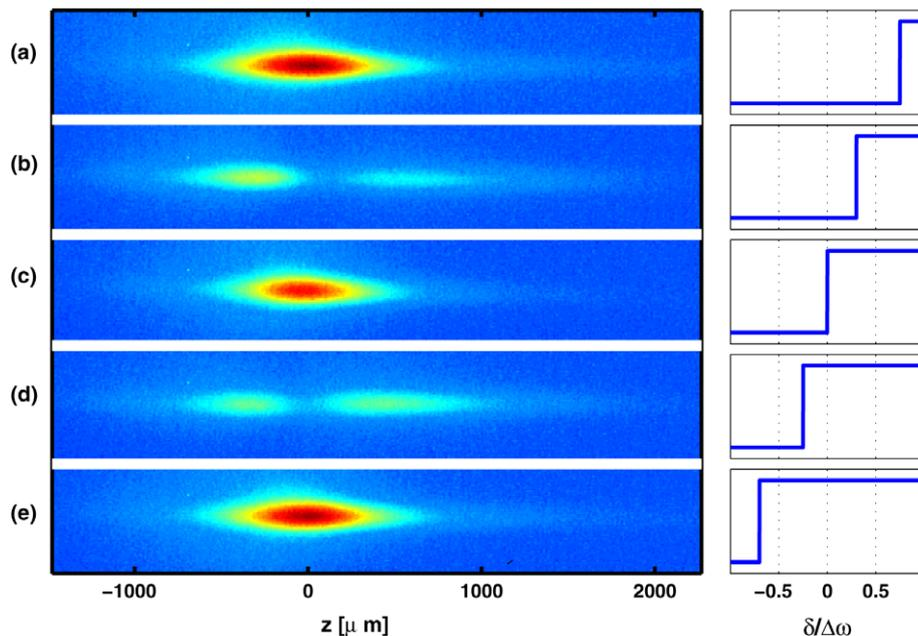
Fig. 3. The effect of a  $\pi$  phase-step on the TPA spatial distribution for several values of the step spectral location  $\delta$ . Shown for each image is a schematic of the spectral phase function applied on the SLM. Images (a) and (e) denote a transform-limited pulse. For  $\delta/\Delta\omega = \pm 0.31$  (b, d) a dark nonlinear focus appears at  $z = 0$  for  $\delta = 0$  and (c) the transform-limited result is reproduced.
