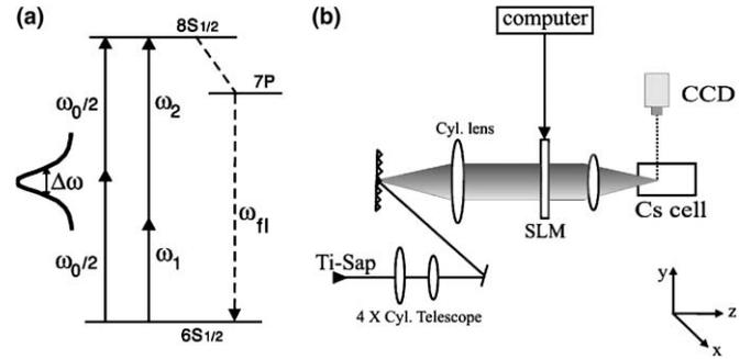
Fig. 1. (a) Schematic diagram of the energy levels of the  $6S_{1/2} - 8S_{1/2}$  two-photon transition in atomic Cs. The excited state population amplitude is monitored by observing the spontaneous decay to the ground level through the  $7P$  level. (b) The experimental setup, see text for details. The coordinate system is showed at the bottom right.
