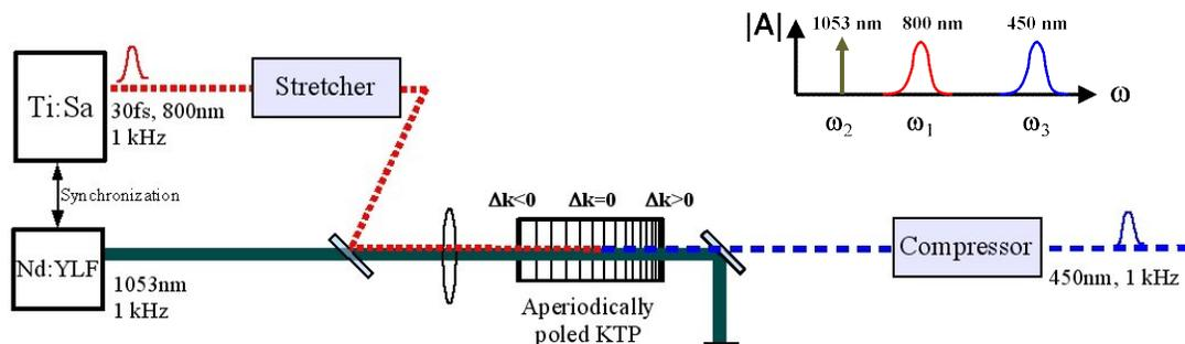
Fig. 1. Implementation of adiabatic frequency conversion of ultrafast pulses. The stretched seed pulse from a Ti:S multipass amplifier (dotted line) and a strong 1053 nm pump beam from a Q-switched Nd:YLF laser (solid line) are mixed in the adiabatic aperiodically poled KTP crystal. Under appropriate adiabatic design of the crystal, the energy of the seed beam is efficiently converted to the sum frequency beam (long dashed line).
